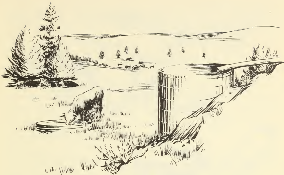
Figure 2.—Water level in a semipermanent stock tank filled from a large storage tank is regulated by a float valve. Gravity feed through a large pipe from truck to storage tank saves time and equipment.
